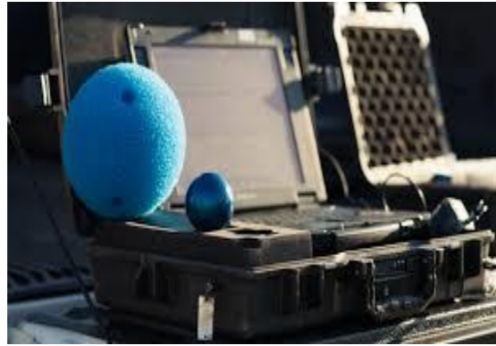
Smartball leak detection
