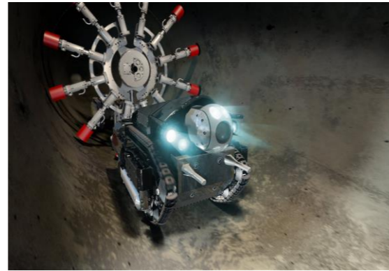
Robotic crawler pipeline inspection
